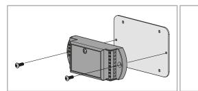
**01.** Secure the module on the plate.
