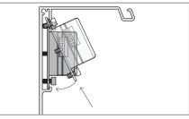
**02.** Place the plate on the door, first engaging the top and then the bottom limits of the plate.
