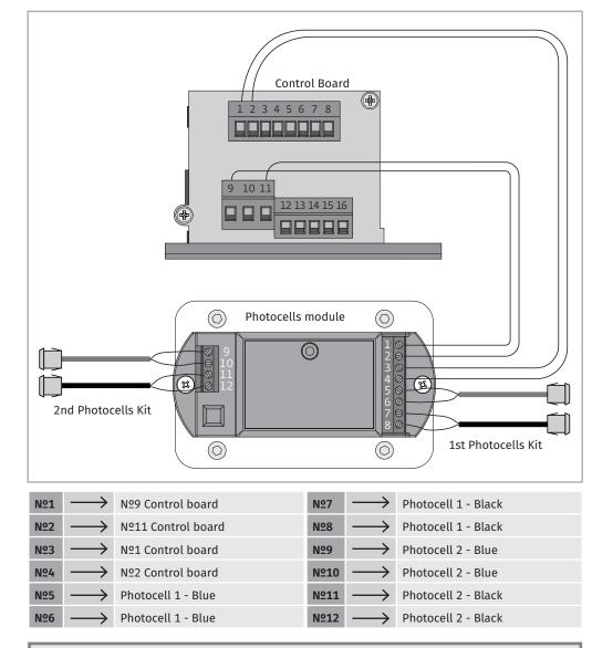
If you install only one photocell kit, you should always connect it on the inputs 5,6,7 and 8.
