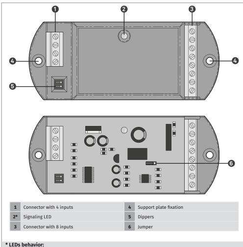
Red (Fixed) - In Communication | Green (Fixed) - Photocell interrupted | Green (flashing) - connection error
