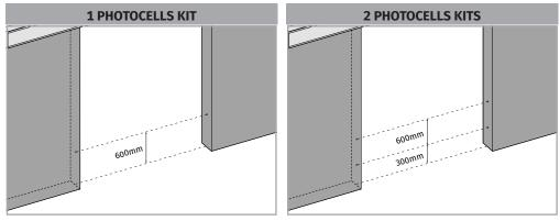
**01.** Measure and mark the drilling holes on the pillars or in the passage's aluminum plates. Note that for proper function, the photocells must be aligned horizontally.
